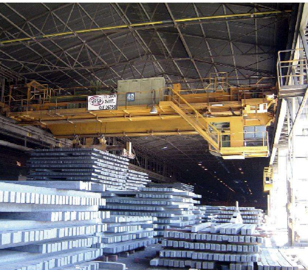
FINISHING PRODUCT E.O.T. CRANE WITH MAGNETS AND REVOLVING CRAB 2X11 T - 18.85 M SPAN.
