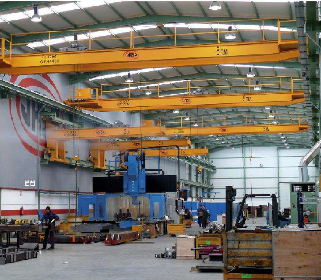
DOUBLE GIRDER CANTILEVER CRANES 2 T - 6 M SPAN / E.O.T. CRANES 5 T - 24 M SPAN.
